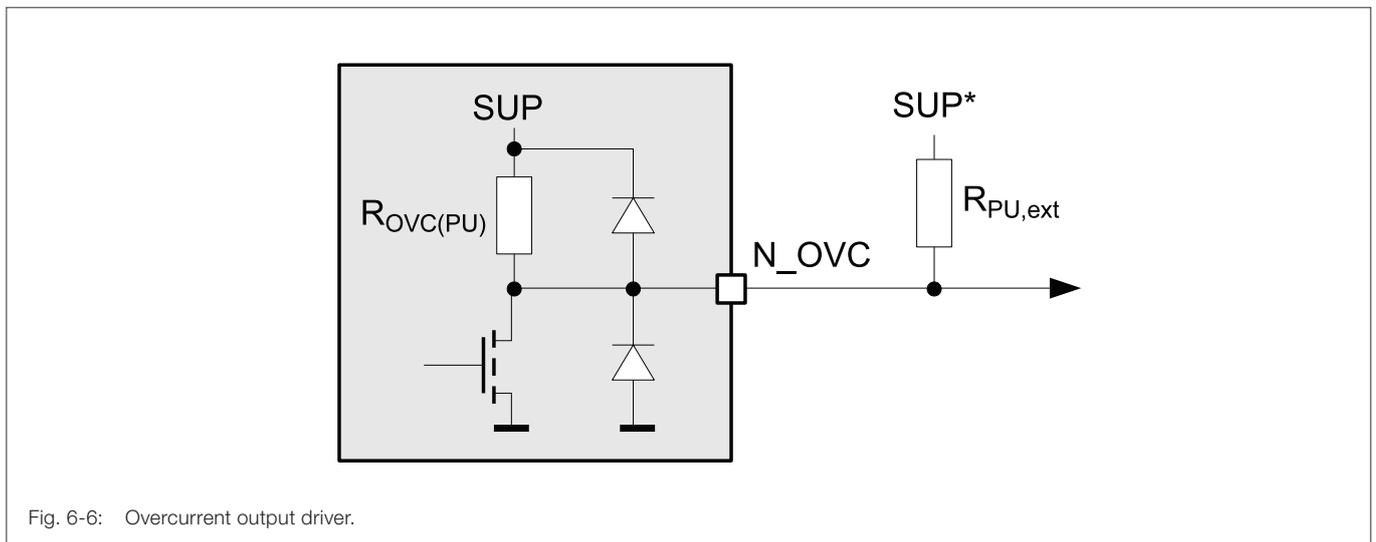
Fig. 6-6: Overcurrent output driver.
