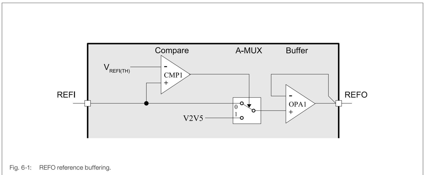
This means, the input REFI is used simultaneously as a reference voltage input and for the level based decision which reference to be fed to the output.
