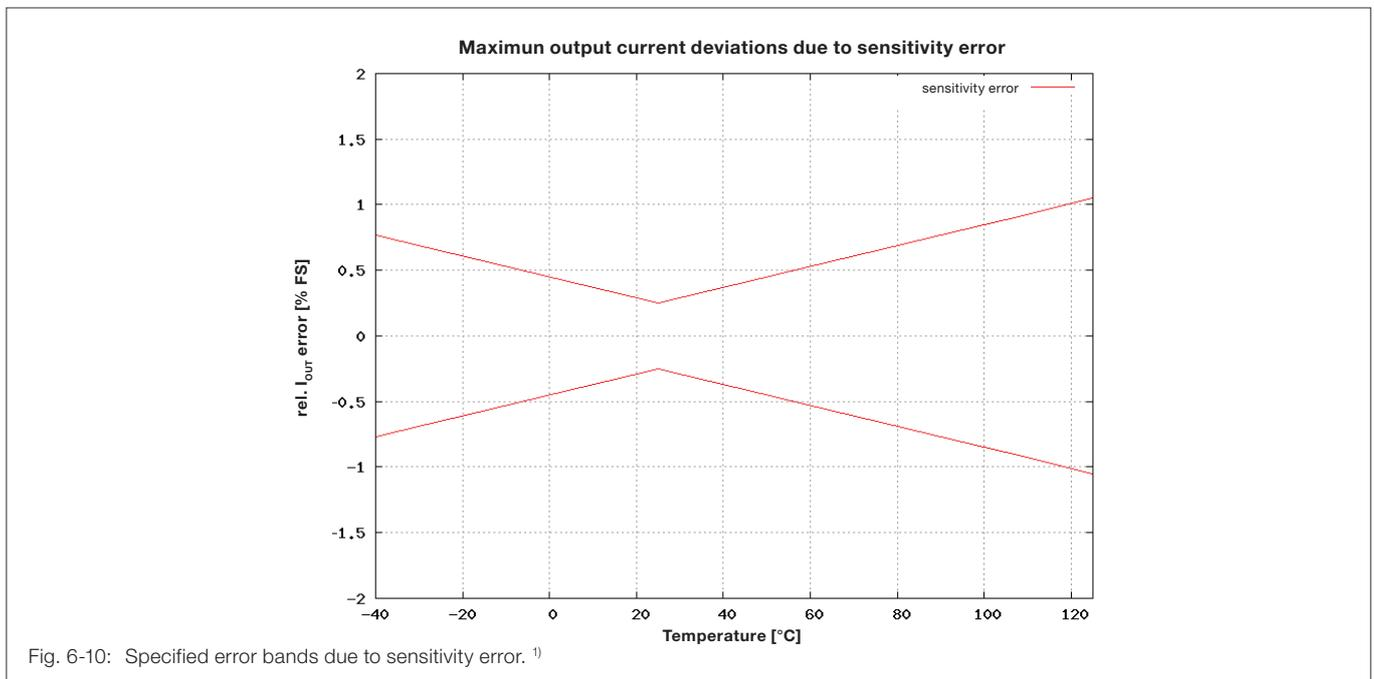
Fig. 6-10: Specified error bands due to sensitivity error. <sup>1)</sup>
