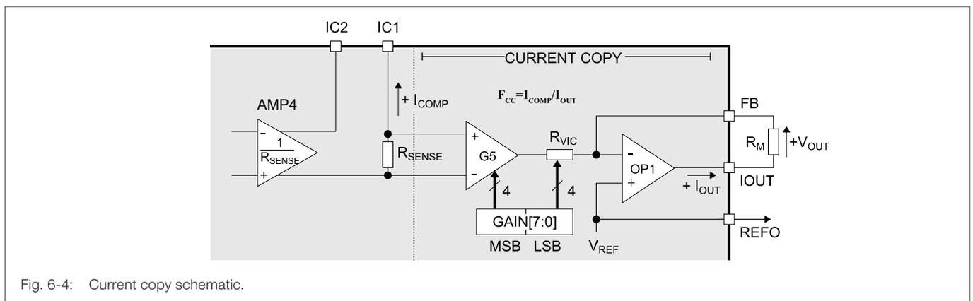
Fig. 6-4: Current copy schematic.
