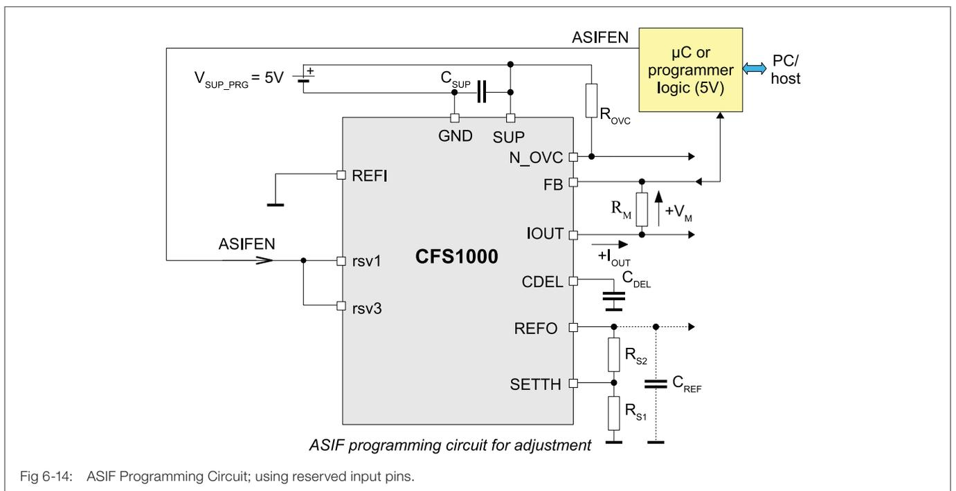
Fig 6-14: ASIF Programming Circuit; using reserved input pins.
