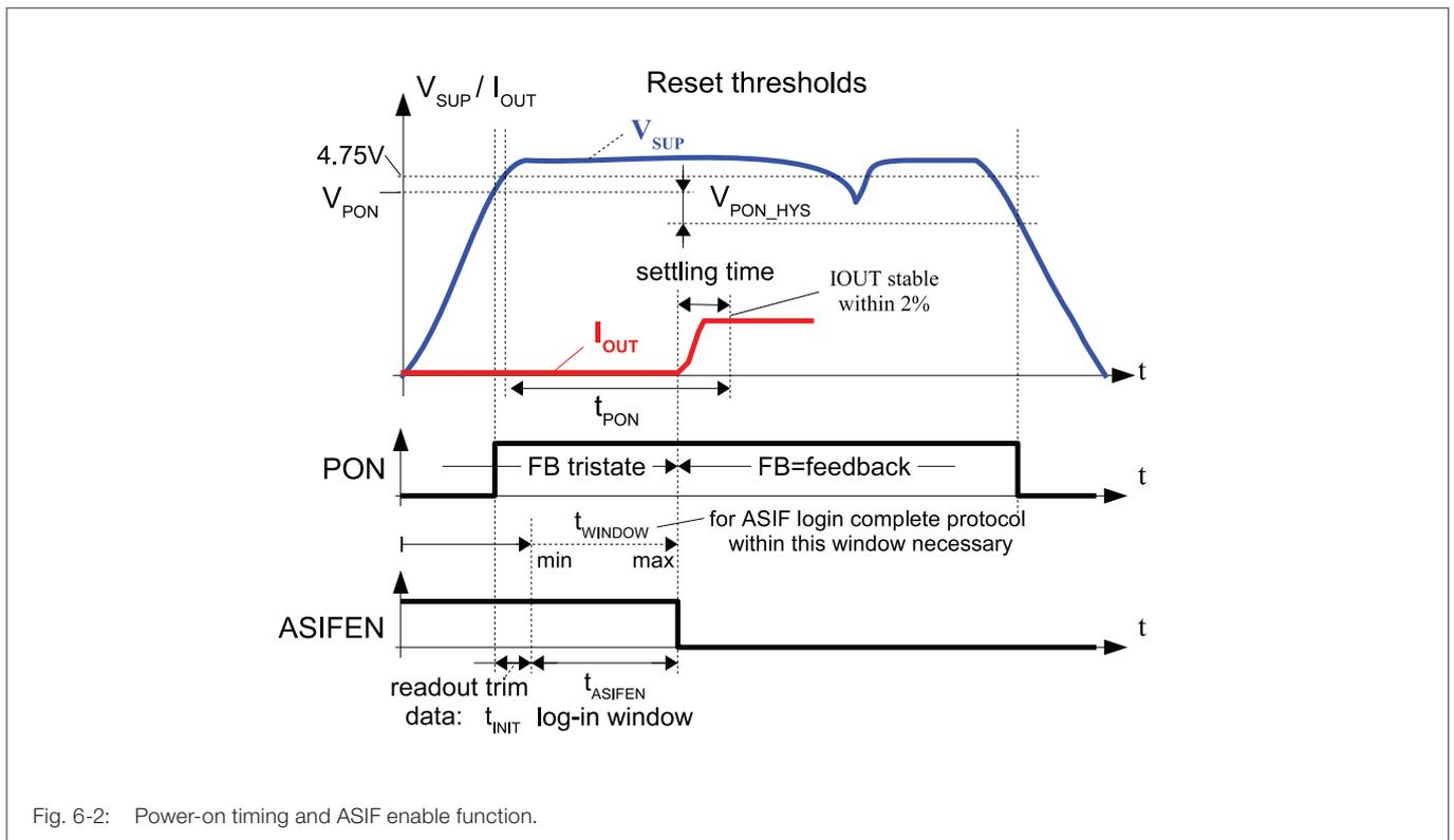
Fig. 6-2: Power-on timing and ASIF enable function.
