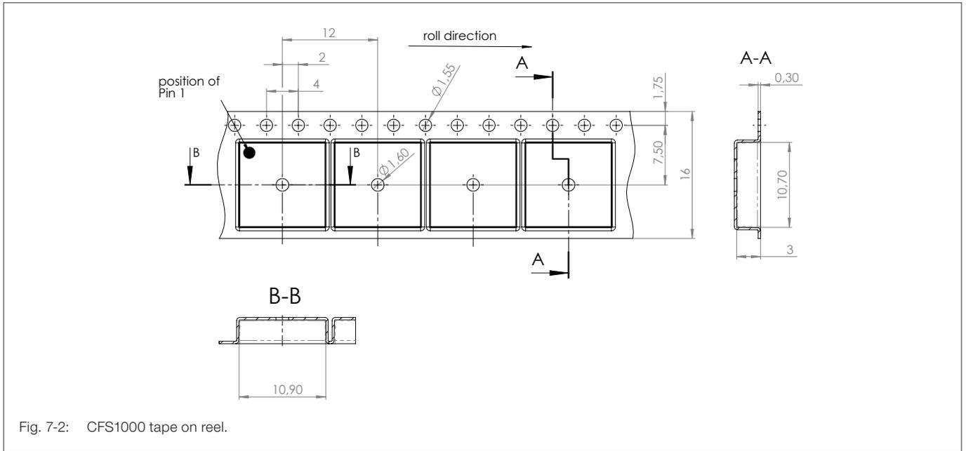
Fig. 7-2: CFS1000 tape on reel.
