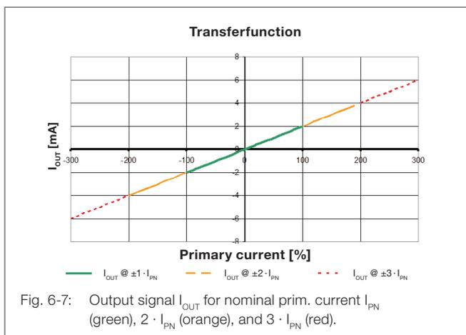
Fig. 6-7: Output signal  $I_{OUT}$  for nominal prim. current  $I_{PN}$  (green),  $2 \cdot I_{PN}$  (orange), and  $3 \cdot I_{PN}$  (red).
