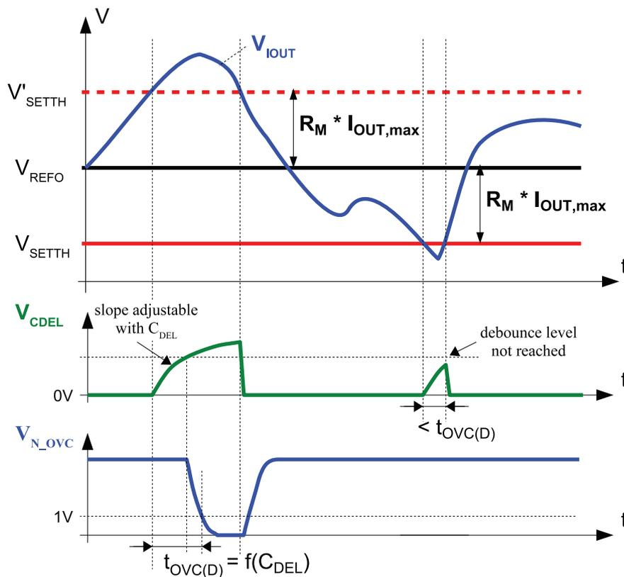
Fig. 6-5: Overcurrent alarm: thresholds and debounce behavior.
