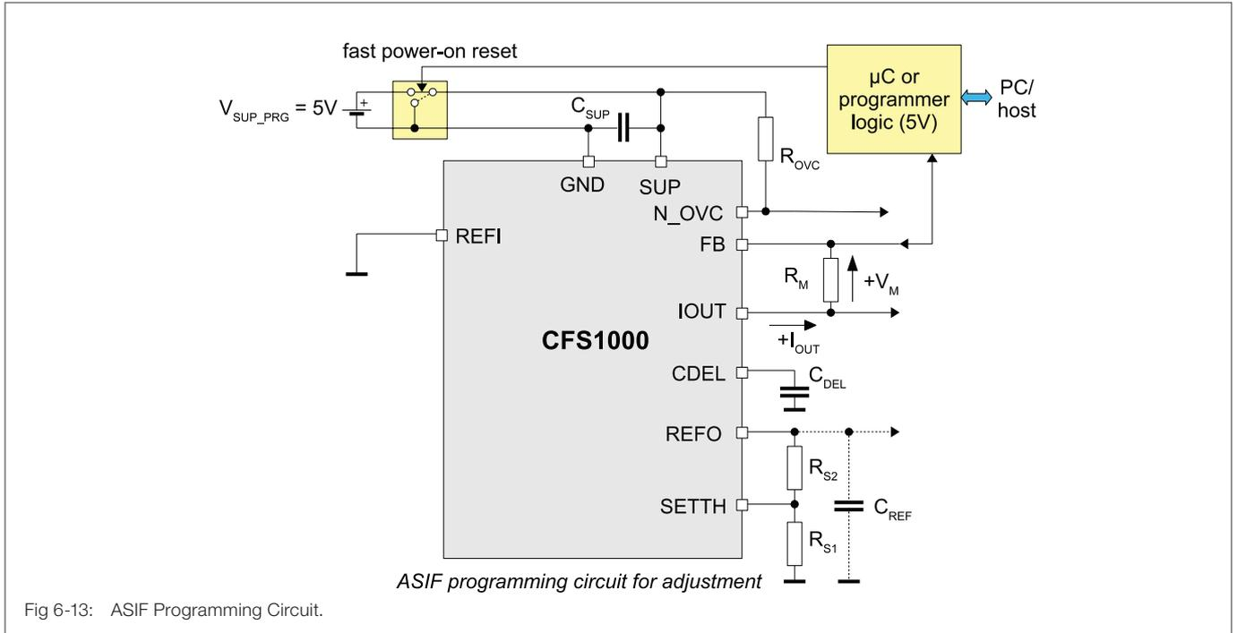
Fig 6-13: ASIF Programming Circuit.
