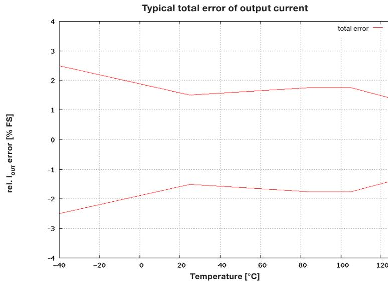
Fig. 6-11: Typical maximum range of total error after calibration. <sup>1), 2)</sup>
