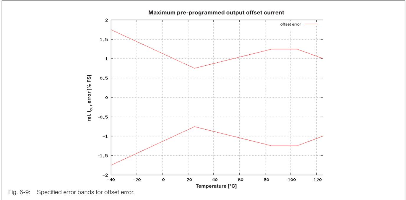
Fig. 6-9: Specified error bands for offset error.
