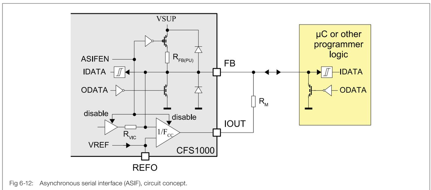
Fig 6-12: Asynchronous serial interface (ASIF), circuit concept.
