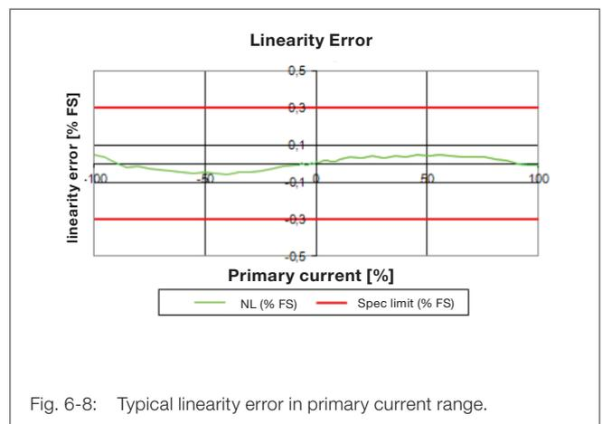
Fig. 6-8: Typical linearity error in primary current range.
