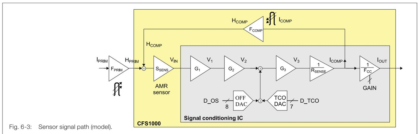
Fig. 6-3: Sensor signal path (model).
