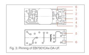
Note: Do not connect a load to the pads 1 and 4 during operation.
