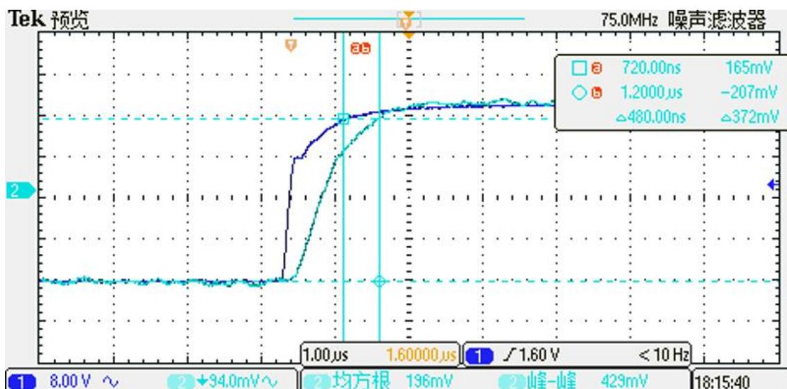
The typical frequency response of STK-616EM current sensor. The response time from 90% of the primary current to 90% of the secondary output is 0.5  $\mu$ s.
