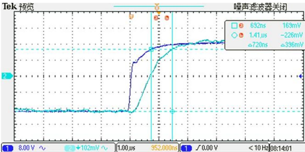
The typical frequency response of STK-616EM current sensor. The response time from 90% of the primary current to 90% of the secondary output is 0.9  $\mu$ s..
