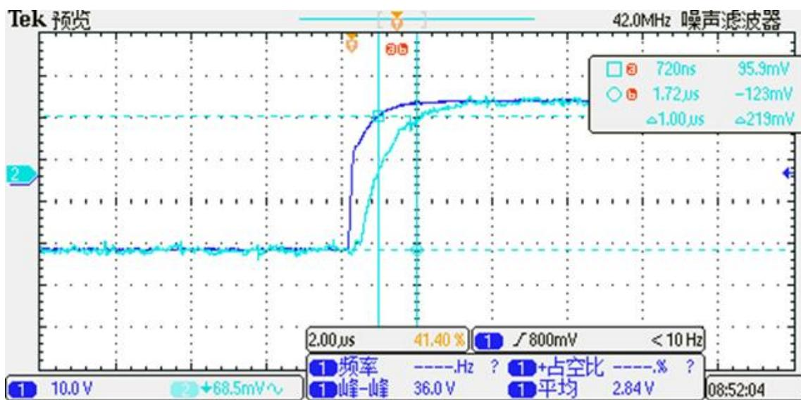
The typical frequency response of STK-616Z current sensor. The response time from 90% of the primary current to 90% of the secondary output is 1  $\mu$ s.
