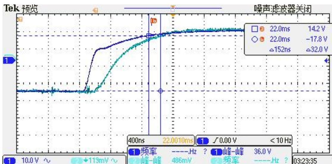
The typical frequency response of STK-616Z current sensor. The response time from 90% of the primary current to 90% of the secondary output is 0.2  $\mu$ s.
