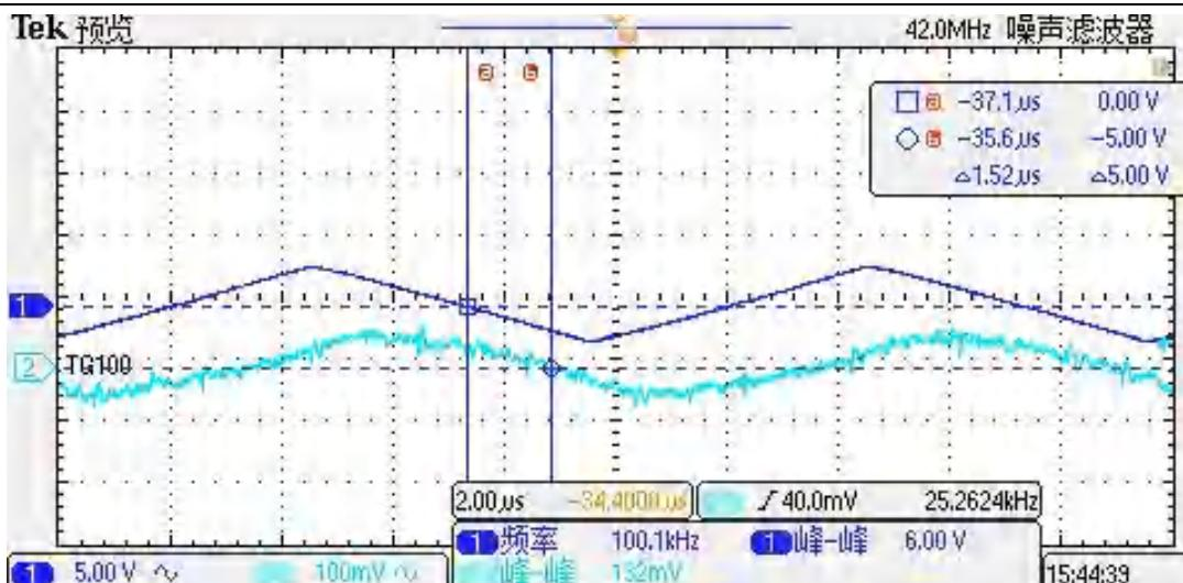
The typical frequency response of STK-616Y current sensor. The delay of output to the primary triangle current with a frequency of 100 kHz is around 1.52us.
