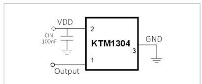
Note:  $C_{IN}$  is for stabilization and to strengthen the noise immunity, the recommended capacitance is 100nF typical and should be placed as close to the supply pin as possible.
