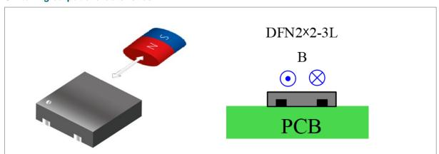
To operate the TMR switch, the magnetic field should be applied to the sensor with sufficient magnetic flux density and correct direction. A horizontal magnetic field parallel to the package can be detected.
